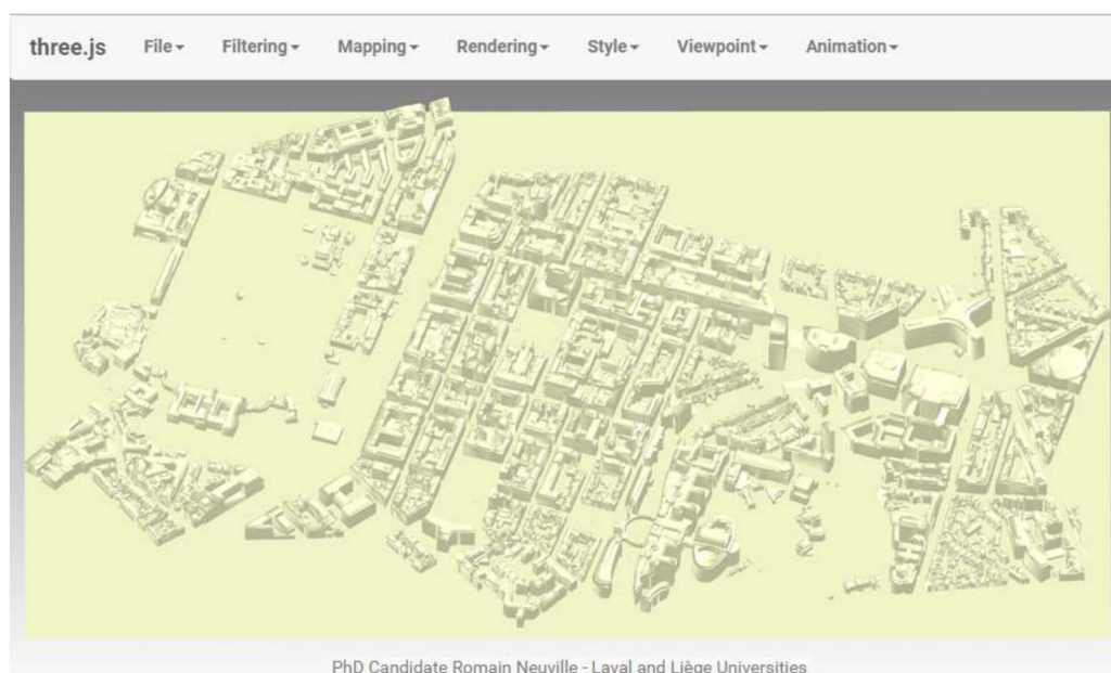
Figure 8. A web application developed as a 3D viewer and including the viewpoint and flythrough creation algorithms (Viewpoint and Animation tabs). The Mapping and Rendering tabs assist the 3D geovisualization process.
