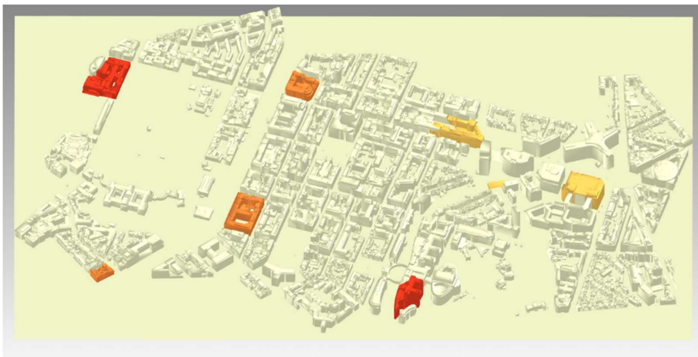
Figure 9. A virtual 3D LOD2 city model of the European Quarter (Brussels). The subway and railway stations are colored from yellow to red, respectively for small to large areas of influence.
